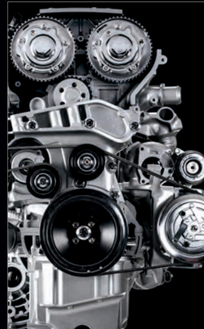
1750 turbocharged, aluminum, 4-cylinder engine
