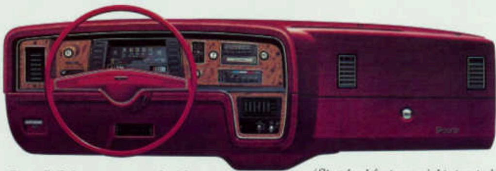
Pacer D/L instrument panel with air conditioning, Entertainment Center, electric clock options.
