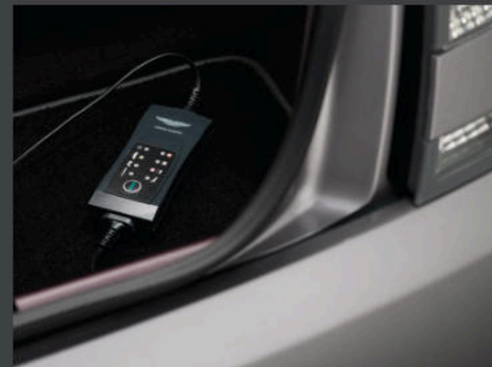
Battery Conditioning Unit
