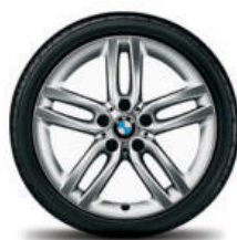
Double Spoke light alloy wheels (Style 461M), 1 18 x 7.5; and 225/40 run-flat 2 all-season tires 3 18 x 7.5 front, 18 x 8.0 rear; and 225/40 front, 245/35 rear run-flat 2 performance tires 3,4
