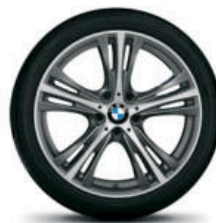
Star Spoke light alloy wheels (Style 407), 19 x 8.0 front, 19 x 8.5 rear; and 225/40 front, 255/35 rear run-flat 1 performance tires 2,3
