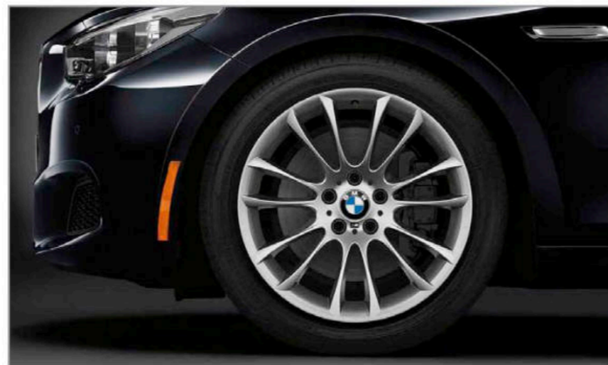
V Spoke light alloy wheels (Style 302M) 19 x 8.5 front and rear; and 245/45 front and rear run-flat all-season tires 1
