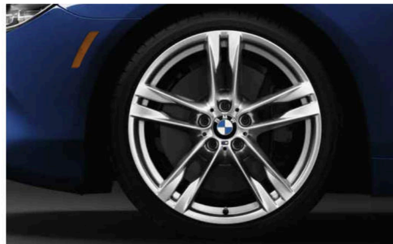
Double Spoke light alloy wheels (Style 373M) 20 x 8.5 front, 20 x 9.0 rear; and 245/35 front, 275/30 rear run-flat performance tires 1, 2, 3
