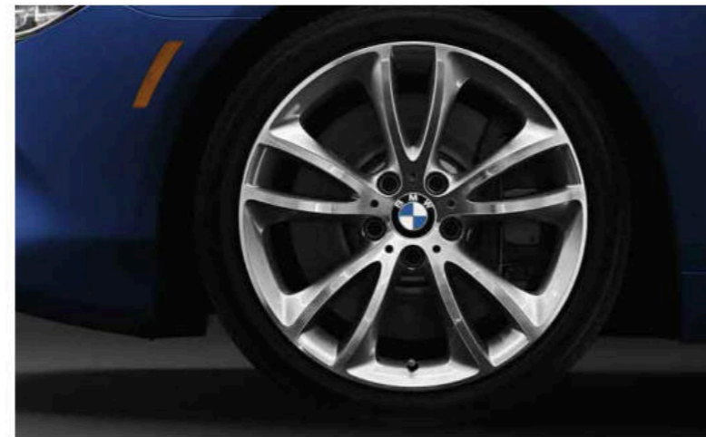
19" V-spoke wheels, style 366, 19 x 8.5 front, 19 x 9.0 rear; and 245/40 front, 275/35 rear performance 1,2 run-flat 3 tires 19 x 8.5; and 245/40 all-season 1 run-flat 3 tires
