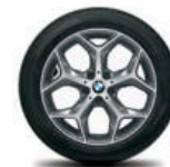
Y Spoke light alloy wheels (Style 569) , 18 x 7.5; and 225/50 run-flat 2 or non-run-flat all-season tires 3
