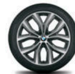
Y Spoke light alloy wheels (Style 511) , 19 x 8.0; and 225/45 run-flat 2 performance tires 3,4
