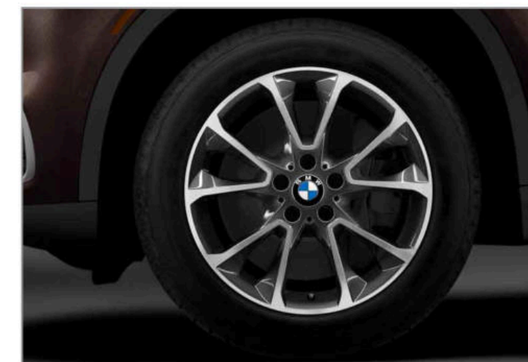
Double Spoke Orbit Gray light alloy wheels (Style 449) 19 x 9.0 front and rear; and 255/50 front and rear run-flat all-season tires 1,2
