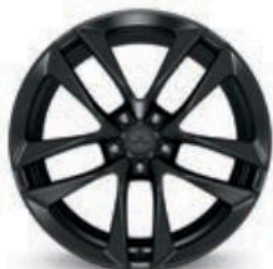
5-Split-Spoke Black-Painted Forged-Aluminum 6 paired with summer-only tires 1 20" x 8.5" Front and 20" x 9.5" Rear on LS or LT
