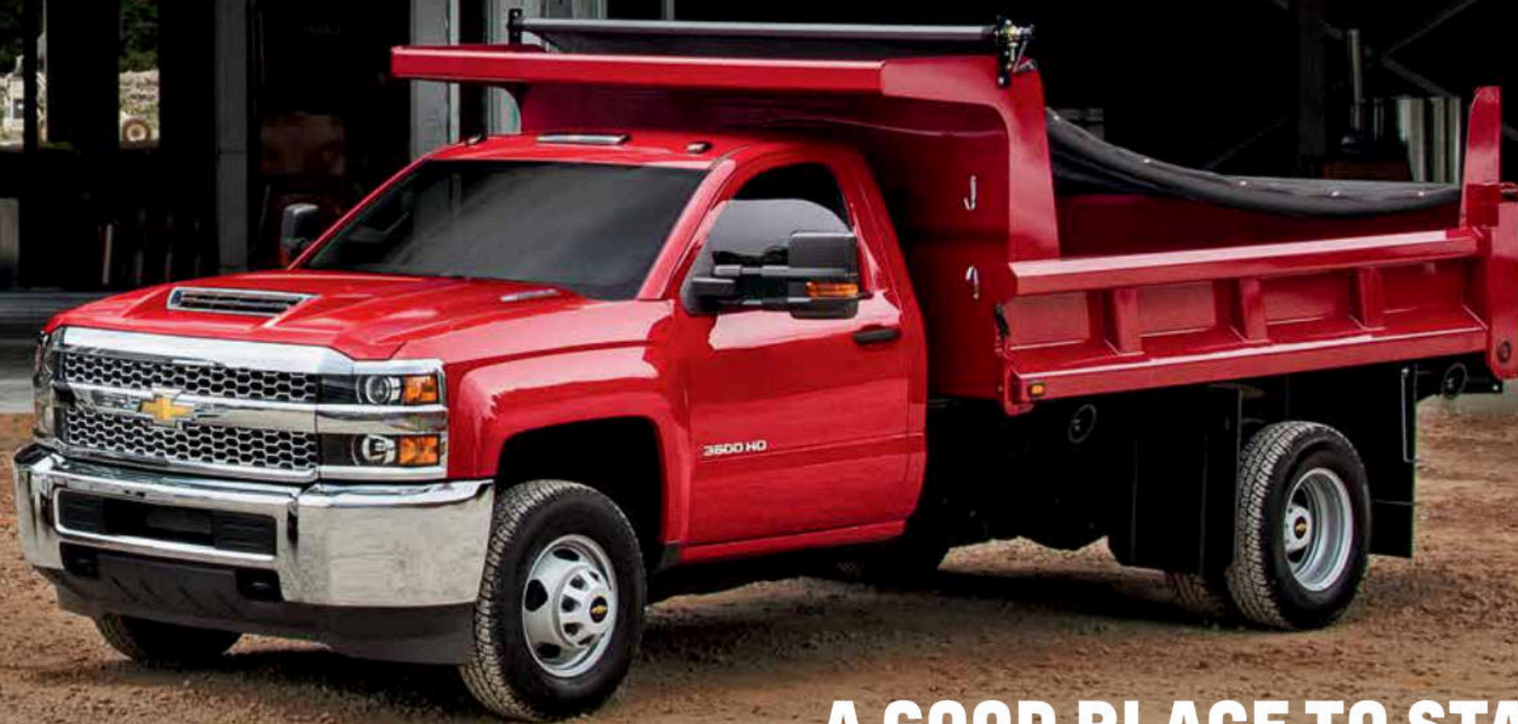
Silverado 3500HD Chassis Cab with a dump body from an independent supplier.
