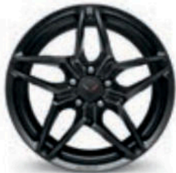
19" x 10.5" Front and 20" x 12" Rear ZR1 10-Spoke Aluminum Wheel in Carbon Flash
