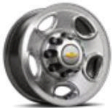
16" Gray-Painted Steel Wheels with Gray Center Caps (QB5); Chrome Center Caps included on 1LT Standard
