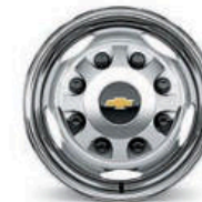
17" Polished Forged-Aluminum (Requires Crew Cab; standard on 3500HD High Country DRW and available on 3500HD LT and LTZ DRW)
