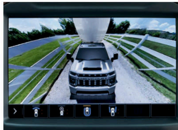
Bowl View Provides a rear-facing 3-D surround view, useful for low-speed backing maneuvers.
