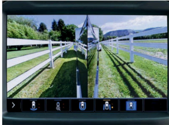
Rear Side View Provides a line of sight down each side of the truck and trailer to provide added views.
