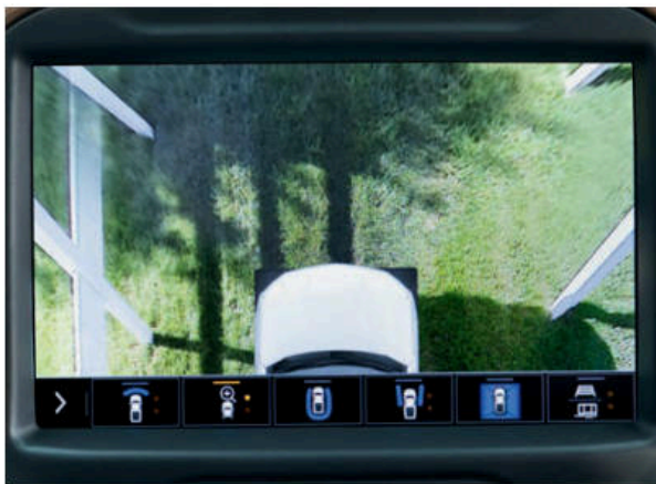
Front Top-Down View A top-down view of the hood, bumper and front tires for tight maneuvers in parking lots or along curbs.
