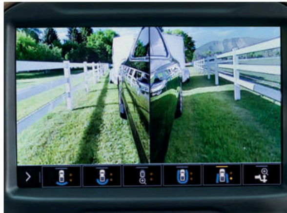
Rear Side View Provides a line of sight down each side of the truck and trailer.
