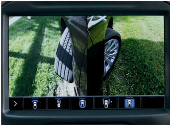
Front Side View Shows the position of the front tires when parking and during tight maneuvers.
