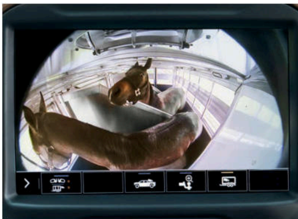
Inside Trailer View Allows the driver to monitor trailer contents or cargo using an available accessory camera that can be installed in the trailer.
