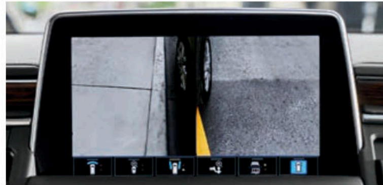
Rear Side View Provides a line of sight down each side of the vehicle.
