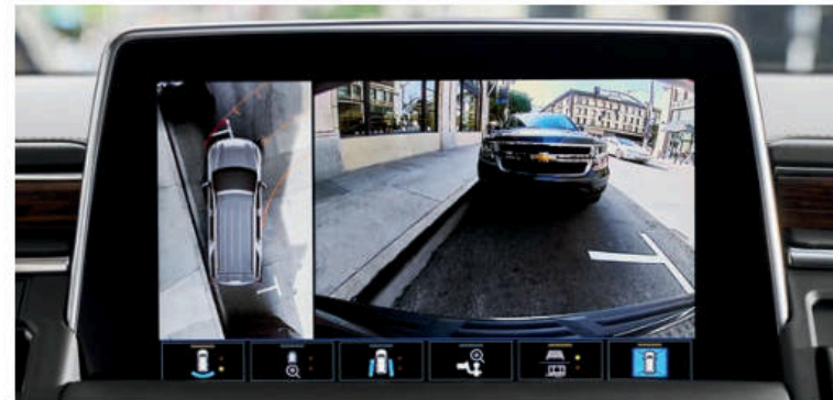
Surround View Gives a top-down bird's-eye view of the vehicle's surroundings.
