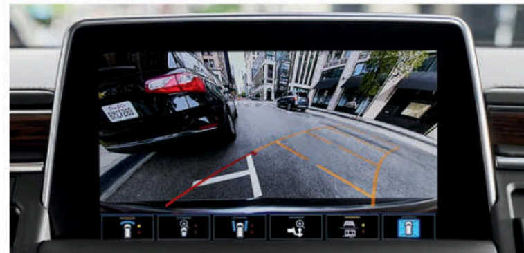
Front Camera View Displays a front view with available guidelines to assist with parking and tight maneuvers.
