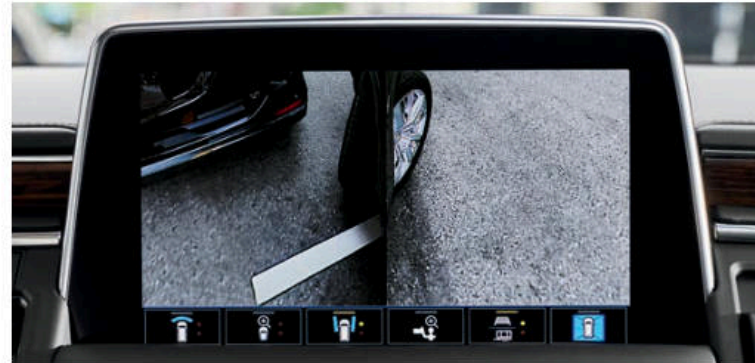
Front Side View Shows the position of the front tires when parking and during tight maneuvers.
