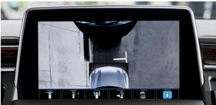
Front Top-Down View A top-down view of the hood, bumper and front tires for tight maneuvers in parking lots or along curbs.
