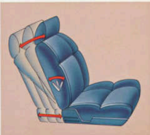
A lever in the seat back adjusts the lumbar support on 510 driver's seat.
