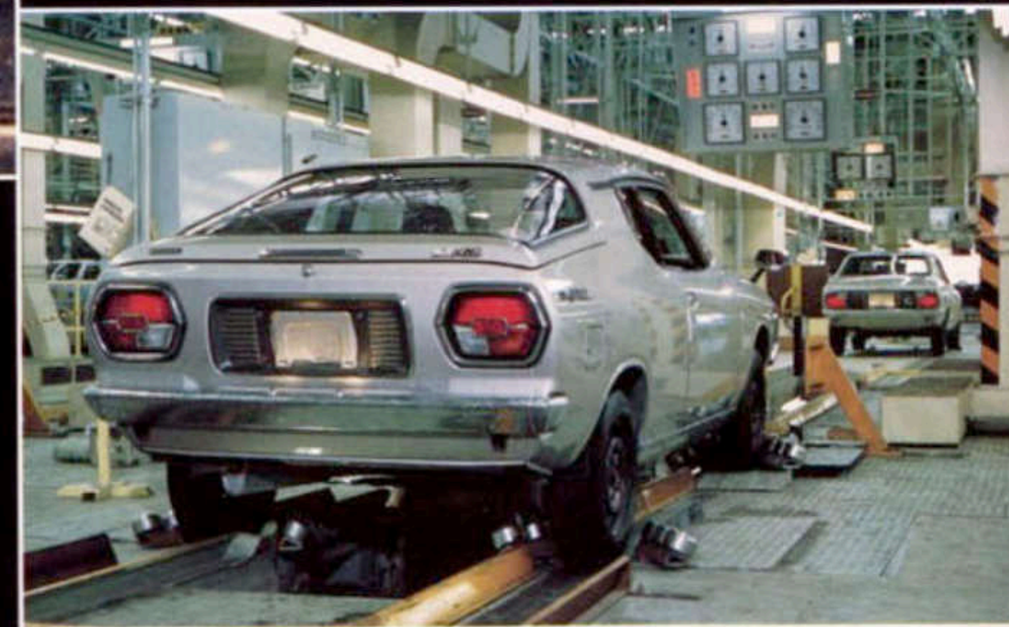
Brakes are tested on dynamometer before vehicle leaves plant. Further brake tests are conducted on test track.
