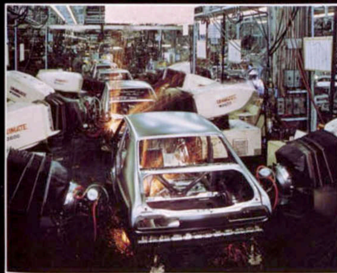
Welding robots are part of automated and computerized assembly line.
