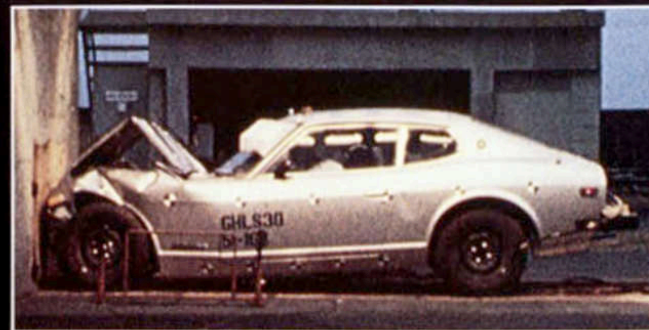
Barrier crash testing helps us determine which parts of Datsun's unibody construction should be rigid and which should incorporate crush zones.
