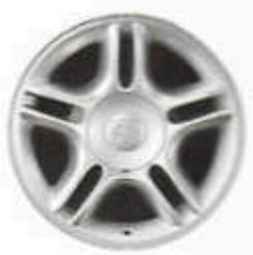
16x8-inch cast aluminum wheel (included with Tire and Handling Group)
