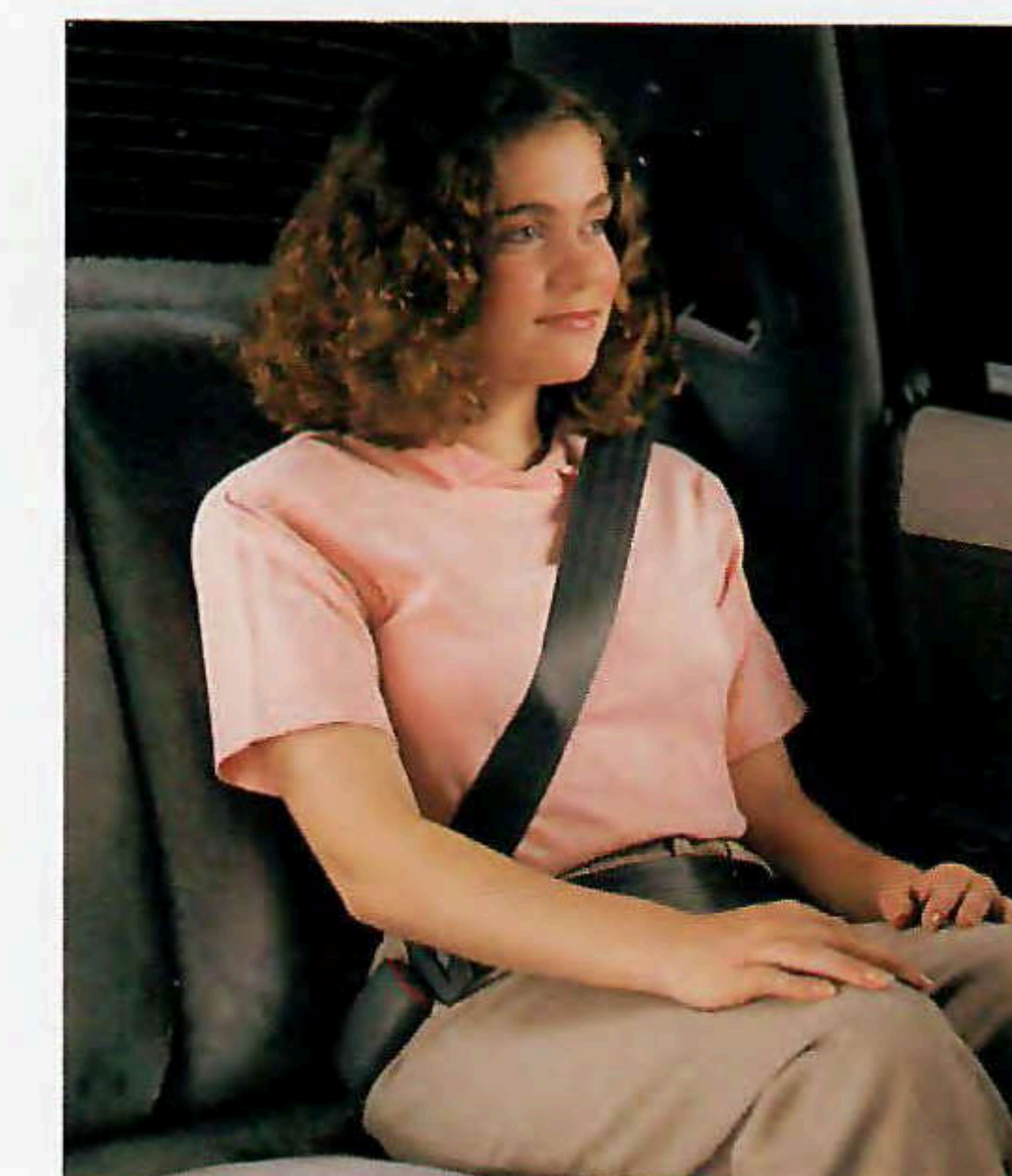
Pillar-mounted Unibelt three-point restraints lock up instantly during severe braking or in a collision, providing outboard passengers with the enhanced benefit of a shoulder restraint.
