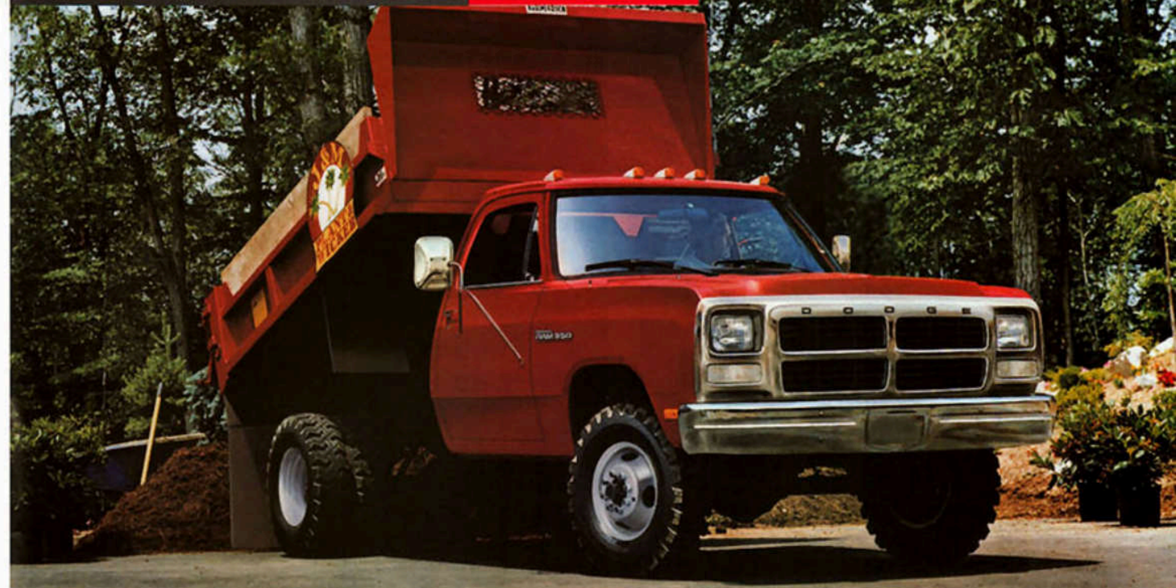
Above: Dual-rear-wheel Ram 350 4x4 with Cummins Intercooled Turbo Diesel shown in Flame Red Clear Coat. The 60-inch cab-axle chassis features a GVW of 11,000 pounds which allows it to easily handle the jobs faced by this three-yard dump body.
