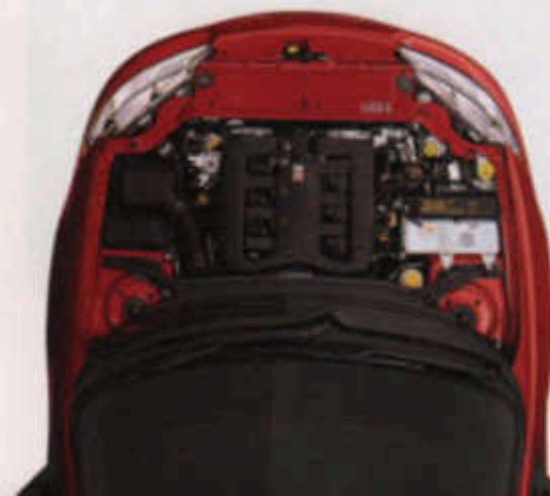
The all-new 3.2-liter aluminum V6 engine, standard on Intrepid ES, produces 225 horsepower and offers 10% better fuel economy than its predecessor.
