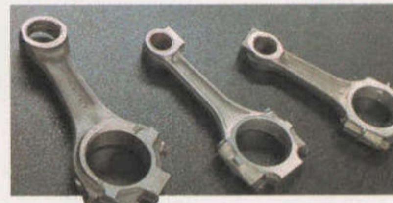
Connecting rods: Dodge Cummins Intercooled Turbo Diesel, Ford Navistar Diesel, Chevy/GMC Detroit Diesel.
