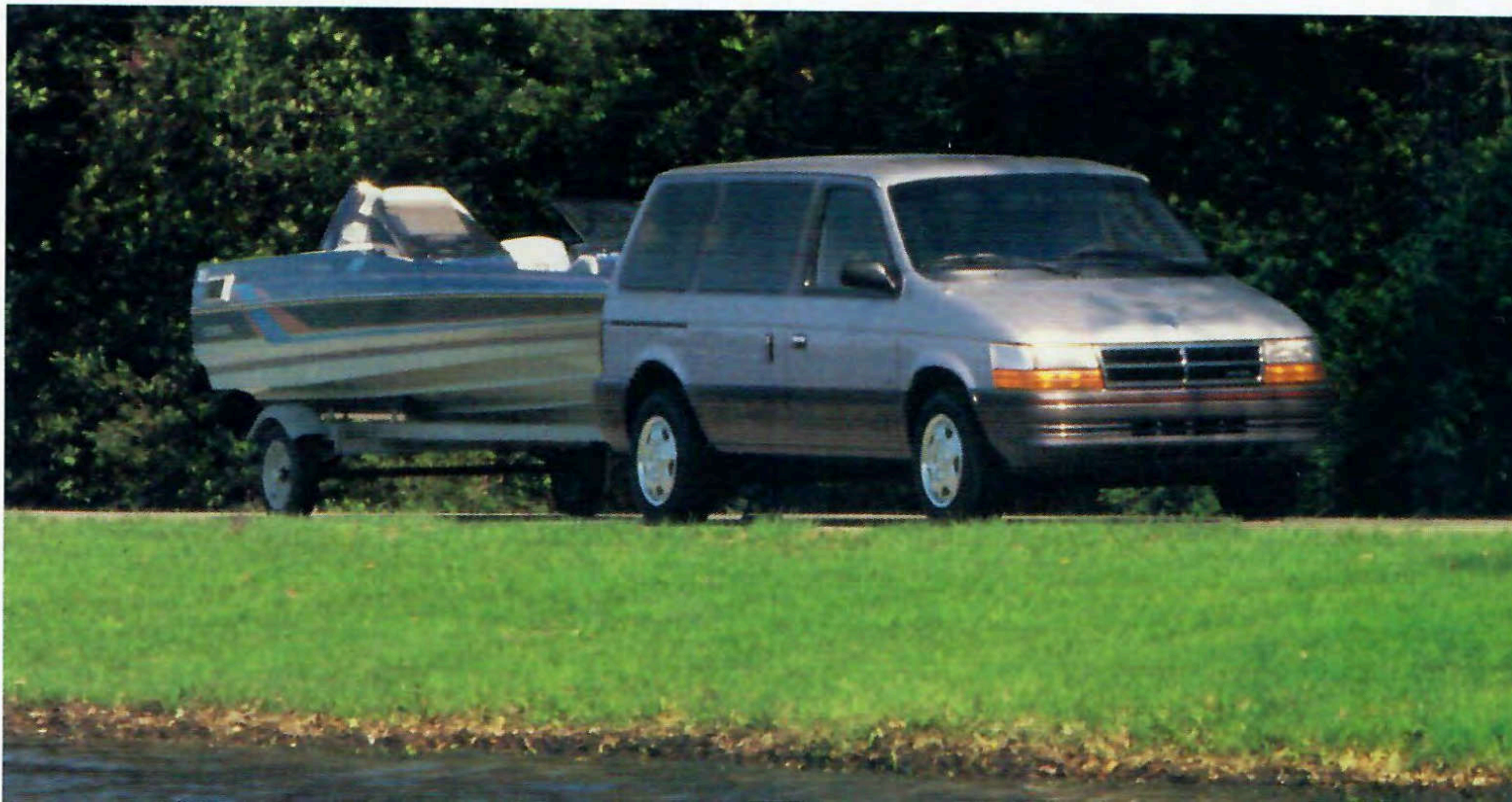
When equipped with the Heavy-Duty Trailer Tow Package and the 3.3-liter OHV MPI V6 engine, the front-wheel-drive Caravan can tow up to 3,100 pounds.
