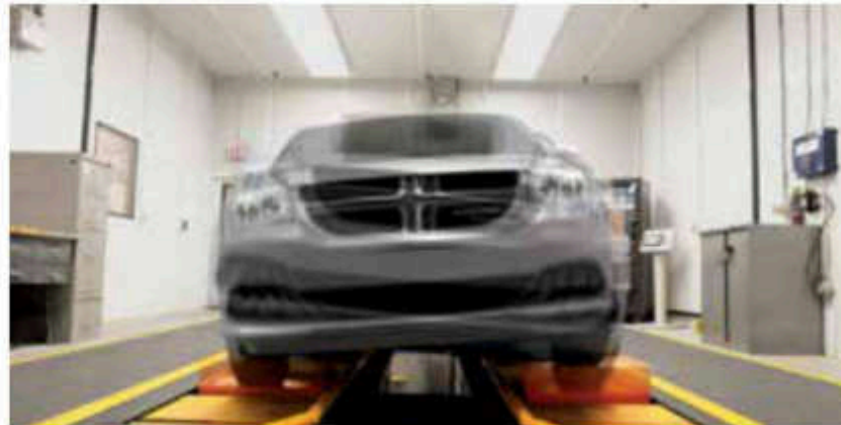
FOUR-POST SHAKER — SUSPENSION TESTING
