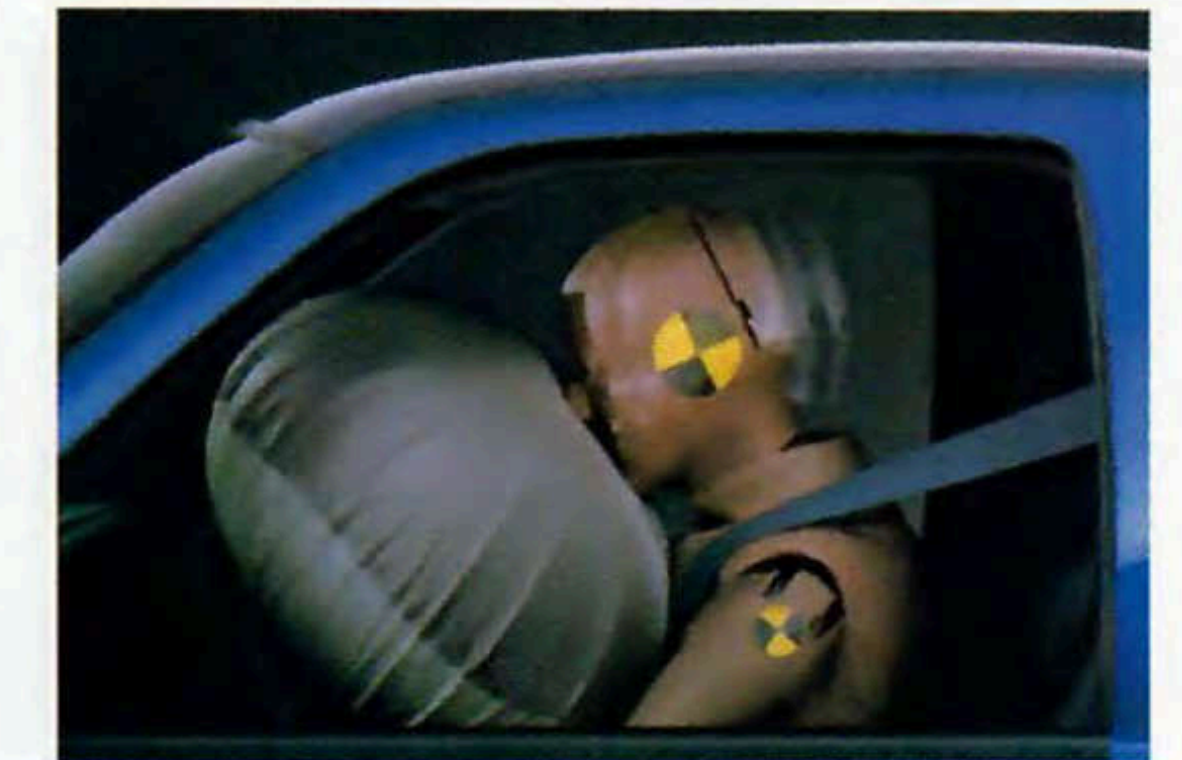
♦ The RAM's air bag* system has been specially engineered to withstand the rigors of real-world truck use. In a sufficient front-end collision, the air bag restraint system inflates, helps protect you, and then deflates, all in a fraction of a second. The RAM's sensing system—which utilizes signals from gold-plated collision sensors in the front fenders and bumper—has been specially tuned to accommodate off-road, snowplowing and towing applications.
