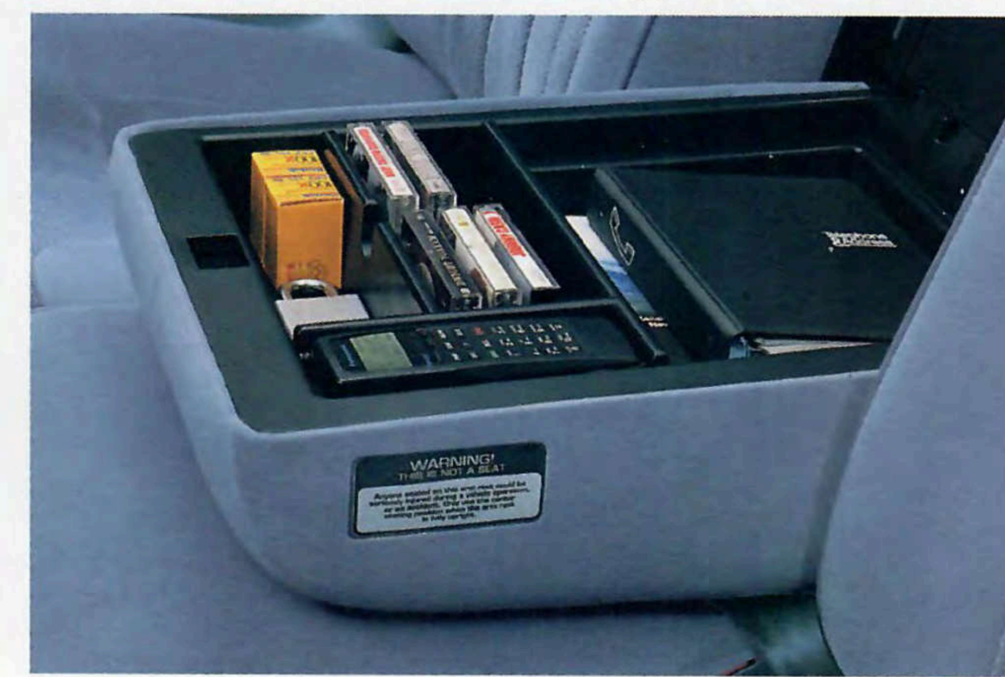
The wide center armrest/console section of the RAM’s 40/20/40 seat (optional on regular cab; standard on club cab) folds down to provide generous storage for cassette tapes, CDs, maps and papers, pens, and much more. The console door’s foam-padded inner surface minimizes the rattling of loose items stored inside.
