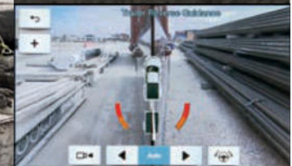
Trailer Reverse Guidance 2 automatically switches between side and rear camera views to show you what is most relevant while backing up your trailer, and provides overlays to guide you.
