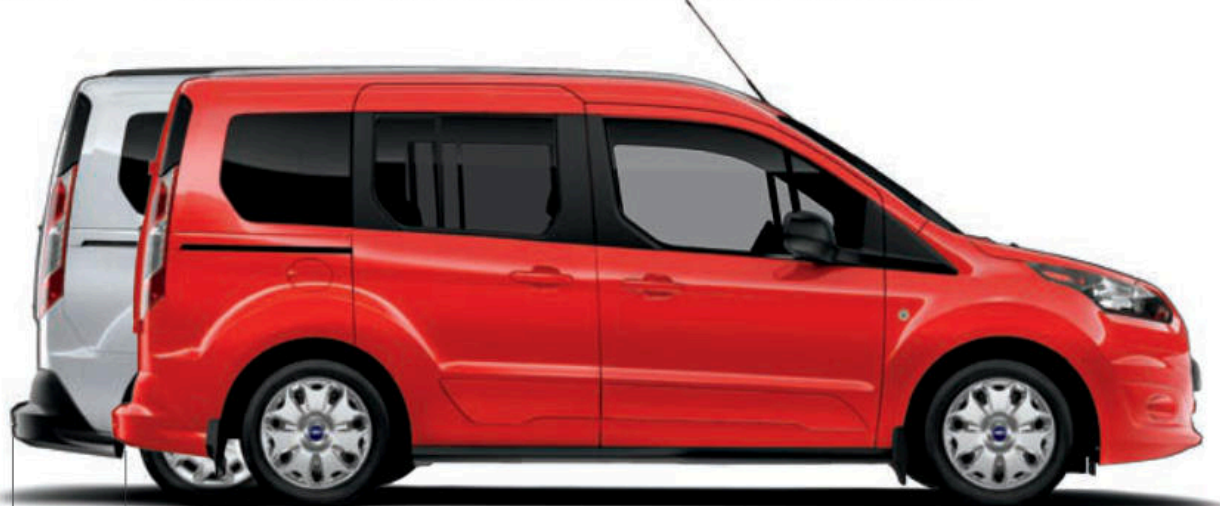
LWB IS 15.8" LONGER OVERALL (LWB) WHEELBASE 120.6" (SWB) WHEELBASE 104.8" (LWB) OVERALL LENGTH 189.7" (SWB) OVERALL LENGTH 173.9"
