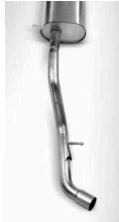
FIGURE 8: CAT-BACK EXHAUST SYSTEM 1
