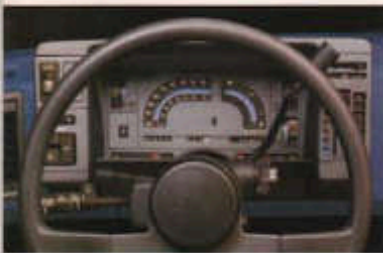
Instrumentation includes a new high-accuracy electric speedometer. Standard full-gauge instrument cluster shown. Electronic gage package with tachometer available.
