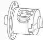
FIGURE 7: FULLY AUTOMATIC LOCKING REAR DIFFERENTIAL
