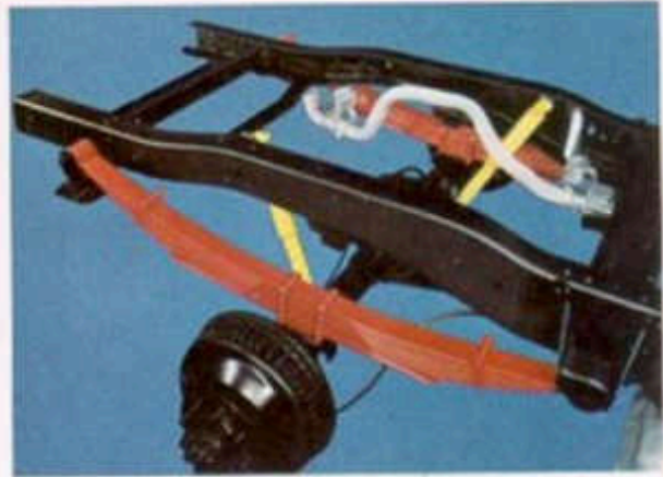
Two-stage leaf spring rear suspension is standard on all light duty models for improved ride control and roll stability. Rear shock absorbers are staggered for improved ride control and to dampen out brake and power hops. Springs and shock absorbers complement each other for improved handling and ride control. New exhaust system hangers permit expansion and contraction of exhaust pipes in operation. New finned cast iron-steel rear brake drums improve cooling.
