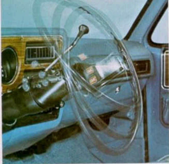
Available Tilt Steering Wheel adjusts to six different positions to suit driver height and seat position. Available with 4-speed manual or automatic transmissions only.
