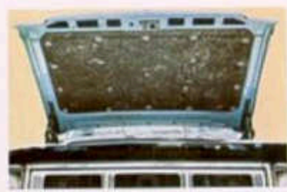
New Hood Design uses dual panels welded together for improved rigidity and reduced hood flutter. Hood insulation (shown above) is available as part of the Sierra or Sierra Grande packages for added sound suppression.
