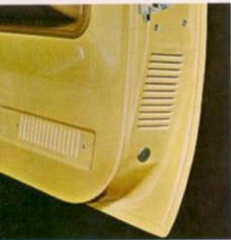
Full Time Power Ventilation on Pickups is standard with outside air supply through a large cowl-mounted plenum chamber. When ignition is on, air is routed through the cab for occupant comfort and exits through door-mounted valves that provide pressure relief when doors and windows are closed.
