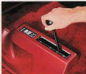
Insta-Trac lets you shift from 2 WHEEL to 4 HIGH and back at any speed.
