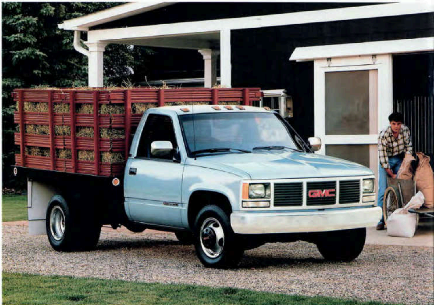
2-WD Series C-3500 SL Regular Cab & Chassis shown with dual rear wheels and other available equipment, including stake rack body from outside supplier
