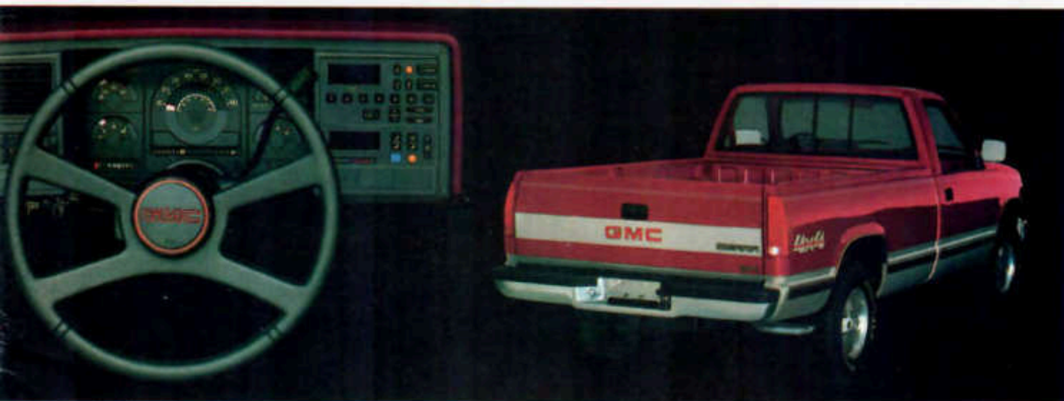
Standard instrument cluster features full gage package and electric speedometer.
