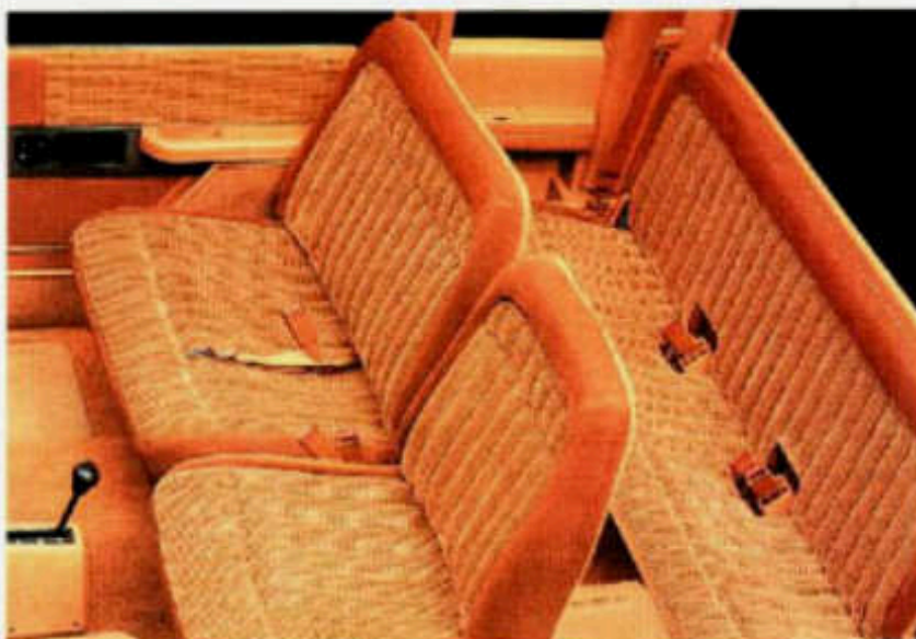
SLE Club Coupe interior with standard front split bench seat and folding rear seat trimmed in Custom Cloth
