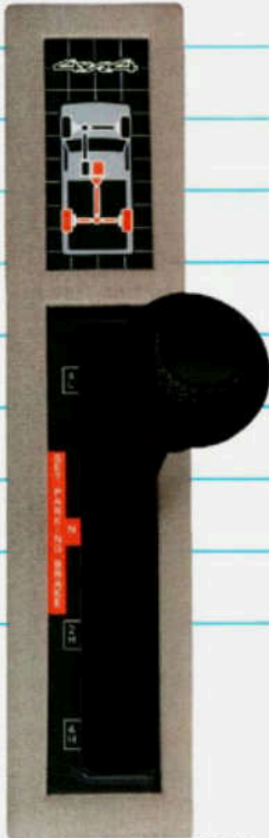
Insta-Trac lets you shift from 2 HIGH to 4 HIGH and back at any speed
