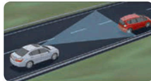
FORWARD COLLISION WARNING (FCW)¹⁰ The FCW system can sense the presence of vehicles in front of you, and if it calculates that you're at risk of a collision with a detected vehicle, it activates audible and visible alerts. (EX-L and above)
