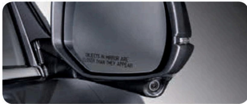
Honda LANEWATCH⁴ A camera under the passenger-side mirror captures more of what's beside and behind you. It displays on your i-MID, revealing more than your mirror can. (EX and above)
