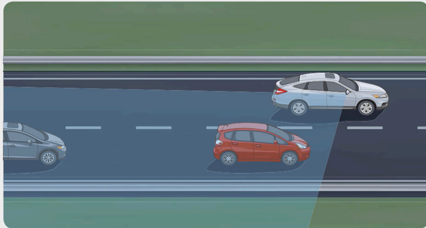
Improve your passenger-side visibility. A lot. Signal right (EX-L and V-6 models) and Honda LaneWatch™ 6 delivers a view to your i-MID that is nearly four times greater than what you would see using the passenger-side mirror alone.
