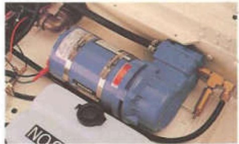
As part of the Central Tire Inflation System, the on-board compressor allows you to inflate or deflate your tires on the move for added traction and a smoother ride in hilly terrain.
