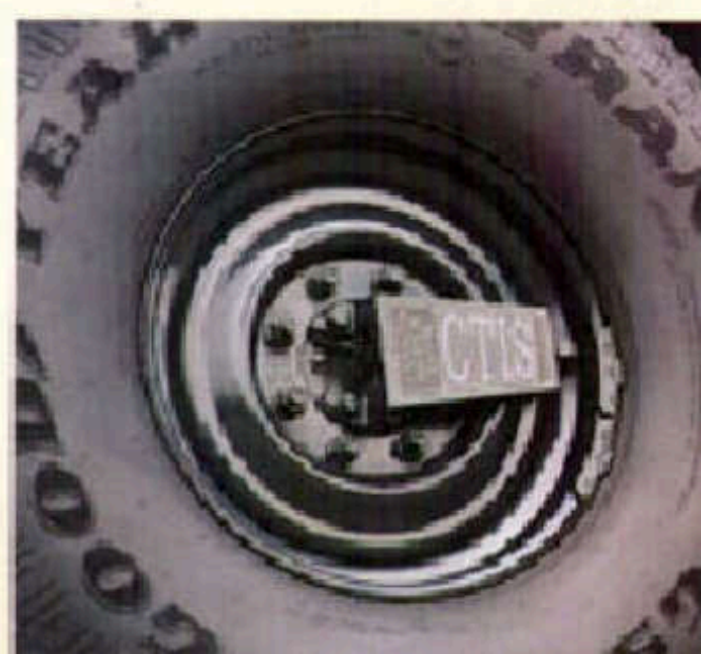
All 1997 Hummers have a lighter, one-piece heavy-duty wheel with runflat and beadlock capabilities.
