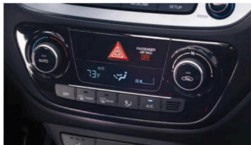
Automatic temperature control
