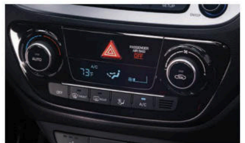
Automatic temperature control
