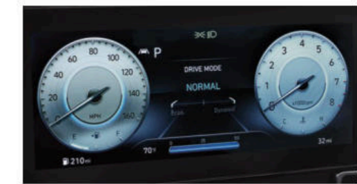
10.25" digital LCD instrument cluster
