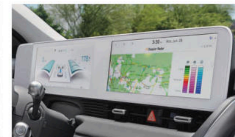
12.3" instrument cluster & touchscreen displays
