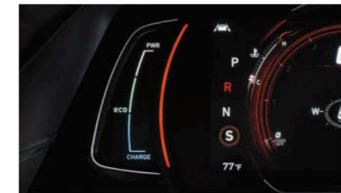
7" LCD instrument cluster – Sport mode
