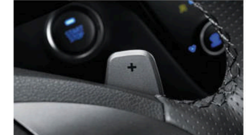
Regenerative brake-level control paddles
