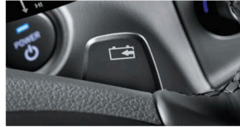
Regenerative brake level control paddles
