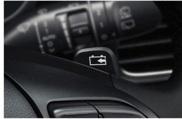
Steering wheel regenerative braking paddles
