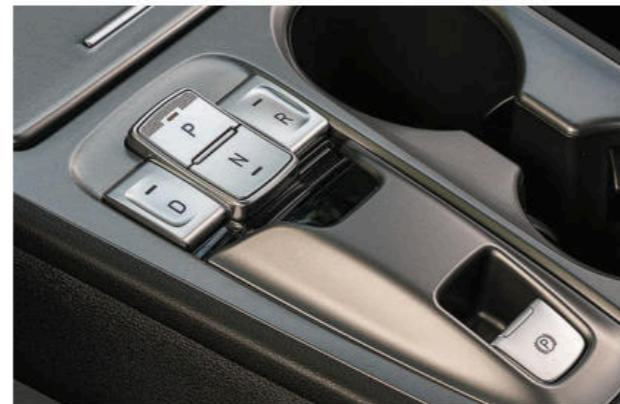
Shift-by-Wire push-button drive controls
